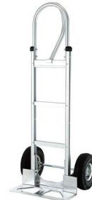
AS16 Loop Handle Size: 52"H x 21"W Weight: 29LB Capacity: 500LB
